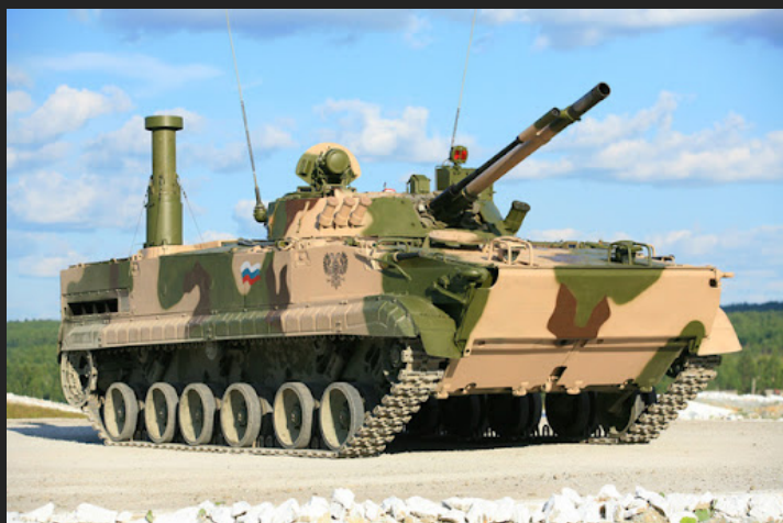
The BMP-3 with 100mm gun and 30mm autocannon prominently displayed.
