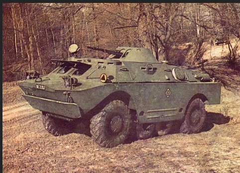
A BRDM-2 conducting reconnaissance. Note the central belly wheels, often retracted.
